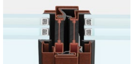
side section | 62 mm visible section
