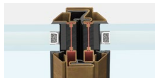
central section | frame section 62 mm
