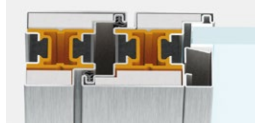
lateral section | frame section 134mm
