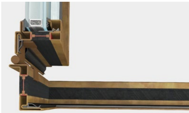
lower section | frame section 47 mm
