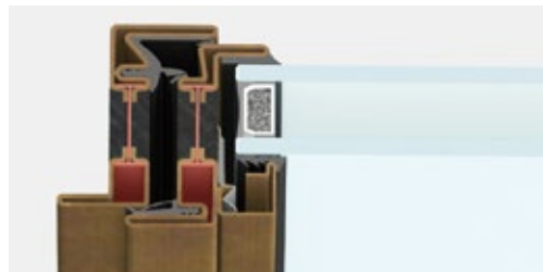
lateral section | frame section 47 mm
