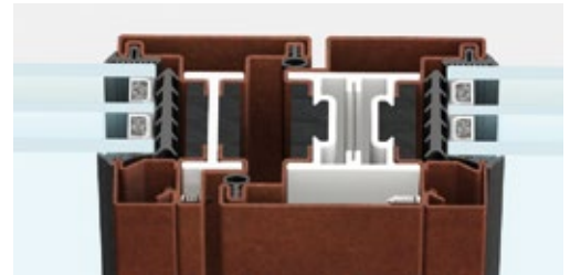
central section | frame section 131 mm
