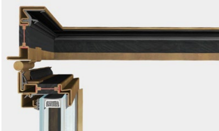
lower section | frame section 47 mm
