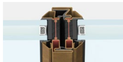
central section | frame section 62 mm
