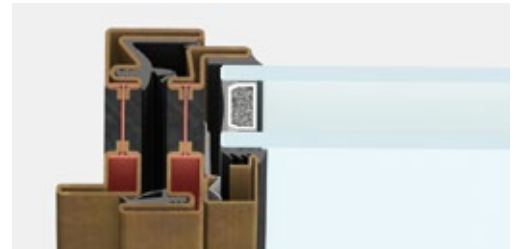
lateral section | frame section 47 mm
