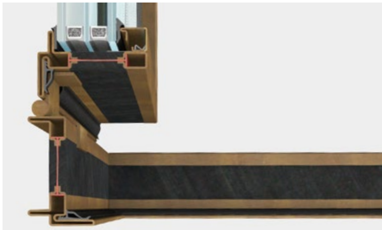
lower section | frame section 47 mm
