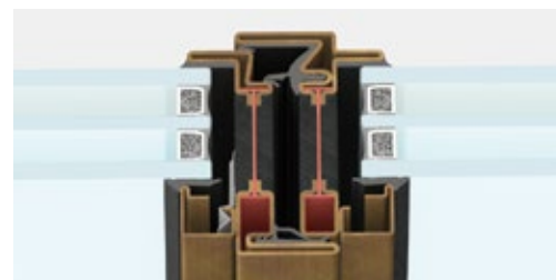
central section | frame section 62 mm
