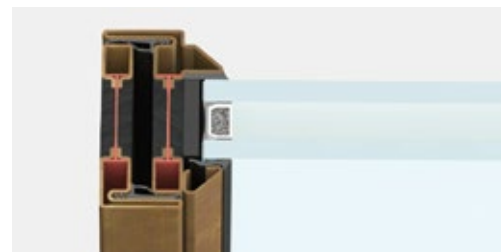
lateral section | frame section 47 mm
