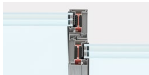
reduced central section | frame section 69mm
