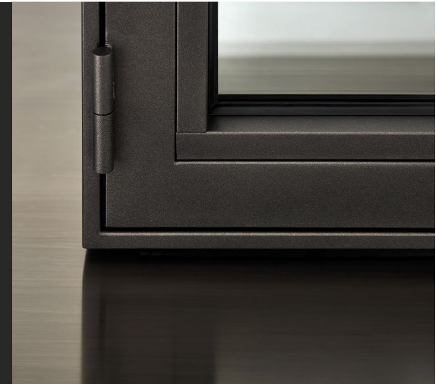
SA 20 window corner, internal view, in painted galvanised steel, sandblasted dark grey colour, with rectangular glazing bead.
