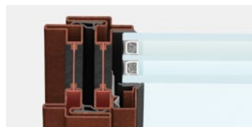
lower side section | 62 mm visible section
