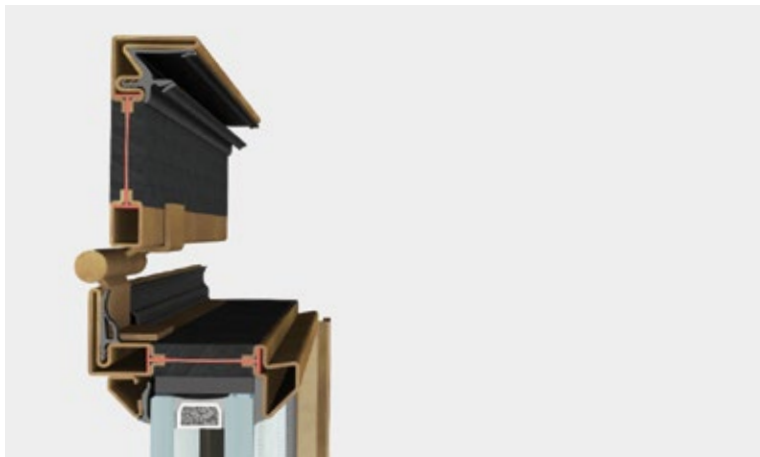
lateral section | frame section 47 mm
